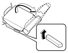
2. Return the seat-bottom to its original position and secure it. After returning the seat-bottom to its original position, make sure the seat-bottom is secured by attempting to lightly move it up and down.
